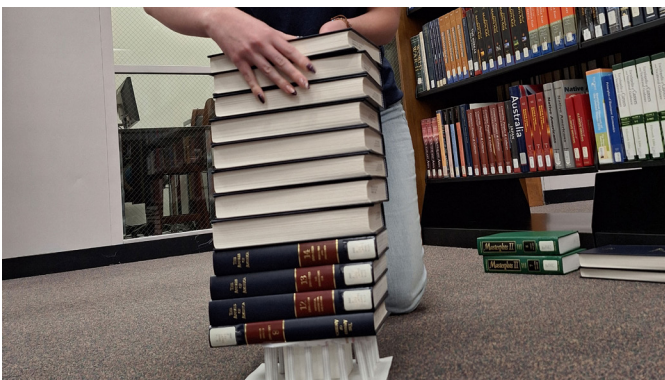
Students stack books on structures made from paper to learn how durable the post-and-lintel system is.
